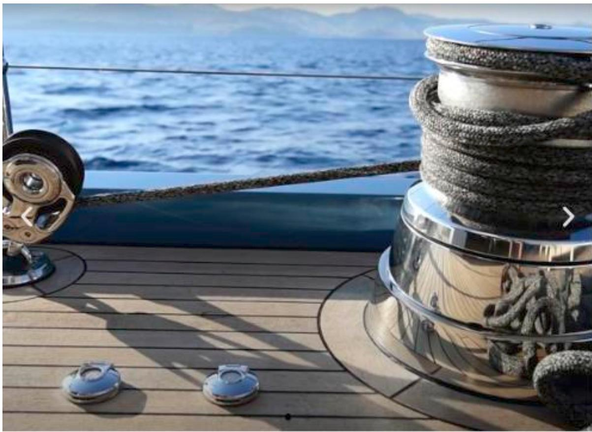
We provide a wide array of sheets. Our ropes construction include 12 plaited core, 24 to 32 plaited covers for the more technical ones.
